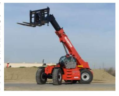
There is also a substantial range of mining attachments, with a fork positioner (width 2,900 mm) with side shift and a capacity of 33 t to 12 m. Designed specially for the high tonnage MHT 12330 telehandler, this positioner assists in the handling of heavy loads used in mines (including spare parts).
