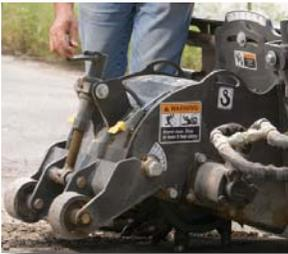
Simple milling depth controls
