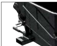
Hitch on forks or on carriage
