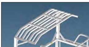
FOPS roof for a maximum protection
