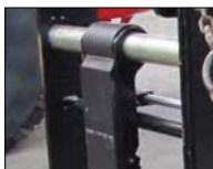
Fork positioning using sliders- forks keep floating
