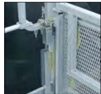
Safety: sensors prevent from platform movements when front part is opened
