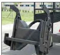
Hydraulic rib clamp- opening 325 - 482mm
