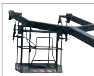
Pendular platform allows work under-bridges
