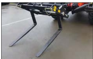
Floating forks with levelling
