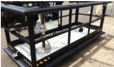
Approach sensors on platform
