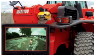
Smart pedestrian detection camera/screen
