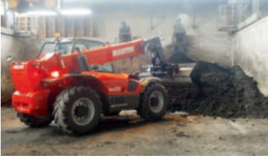
MLT 845: sludge transfer
