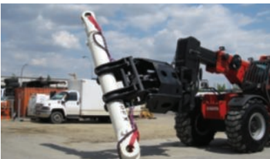
CH10, max capacity 10.5t (23,148lbs)
