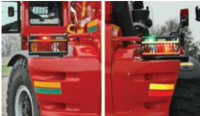
Signal lights for machine approach or withdrawal
