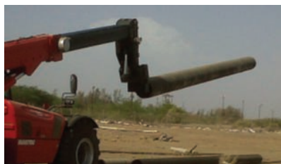
MHT handling a 12m (39.4'), 2.2t (4,850lbs) tube
