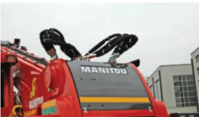
Reinforced synthetic fiber sleeves to protect the hoses
