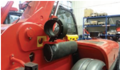
Exhaust gas dilution system
