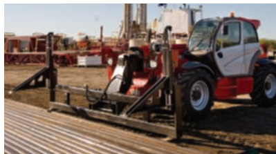
MT and clamp for very long tubes
