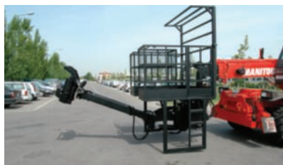
Basket with steel manipulator
