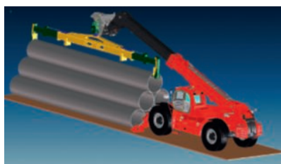
Telescopic rudder on MHT 35t (77,162lbs)
